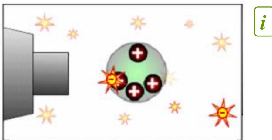
Charge neutralization (corona discharge process)
